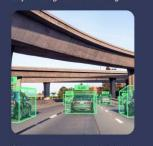
Objects are perceived and identified with image recognition, then velocity/ direction determined by comparing size and movement of identified objects across image frames.
