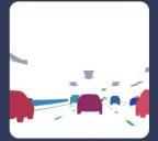
Surfaces that move together over time are grouped into objects (without being explicitly identified), and both stereo vision and pixel expansion techniques are used to determine distance, velocity, direction of motion, and time-to-impact.
